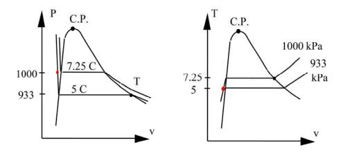
Locate the state of R-410A at 500 kPa,  $-10^{\circ}\text{C}$ . Indicate in both the P-v and the T-v diagrams the location of the nearest states listed in the printed Table B.4
